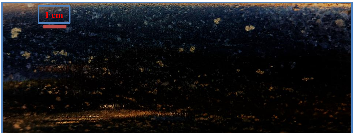
Figure 1. Extensive pyrite in layered gabbro. Note how the sulphide blebs which are up to 0.5 mm in dimension are intergrown with, and are an integral part of, the minerals within the gabbro. These textures are characteristic of magmatic sulphides and extend over a true thickness of about 100 metres.
